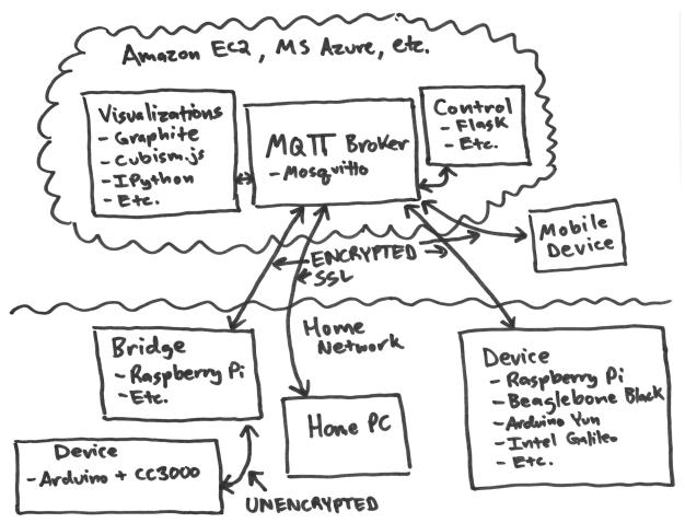
The MQTT broker, mosquitto, is at the center of all communication and lives on a server in Amazon EC2, Microsoft Azure, etc. Along with the broker other applications like visualizations or control apps are hosted on the same server and can communicate with the broker directly.
